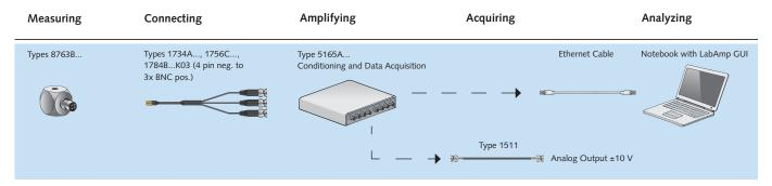
Note: Type 1784B...K03 is used for Type 8763B...A...; Type 1756C... and Type 1734A... are used for Type 8763B...B... and Type 8763B...CBsp
